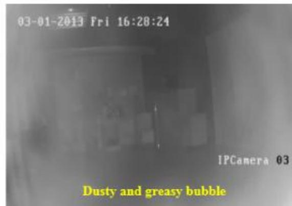
Always clean the dome cover with a soft cloth after installation. Commonly, the domes get covered with dust/dirt, raindrops stains, and cobwebs over time. This will cause the image quality to degrade over a period of time (“foggy condition”). Periodic cleaning of the dome cover may be required to maintain a clear picture.
